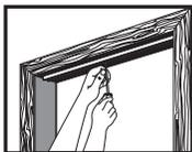
After making a screw pilot hole (with a nail or 3/32" drill), drive a 1" track screw through the screw hole nearest the center of the track. Do not tighten. (Tape may be used to hold the track in place while you mark and drill.)
