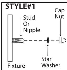
**STYLE#1**- Tuck electrical wires into outlet box and position fixture over studs or nipple on mounting bracket assembly. Secure fixture in place with star washer(s) and cap nut(s).
