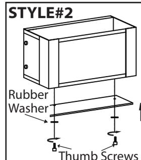
**STYLE#2**- Install proper bulb type and wattage. Secure the glass in place using the rubber washers and the 2 thumb screws.
