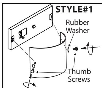
**STYLE#1**- Install proper bulb type and wattage. Secure the glass in place using the rubber washers and the 2 thumb screws.
