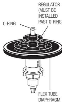
Optima Plus Valve Models Feature Sloan's Exclusive Flex Tube Diaphragm™ for the ultimate in valve performance, reliability and Chloramine resistance.
