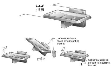
**Mounting of Product:** Screw concealed mounting system: The mounting bracket is attached to the wall with screws at the desired height. The unit is then hooked onto the bracket. When the set screw is tightened the product is firmly secured to the wall. The set screw applies pressure to an inclined surface on the bracket this provides a rattle free and integral mounting of the product. (mounting bracket and screws provided).
