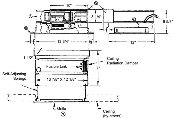
**Note:** Zephyr and CFD-20-DDA6 ceiling radiation dampers are shipped in separate cartons for joining through field installation.
