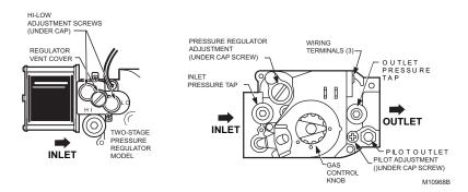
Fig. 6. Top view of gas control.
