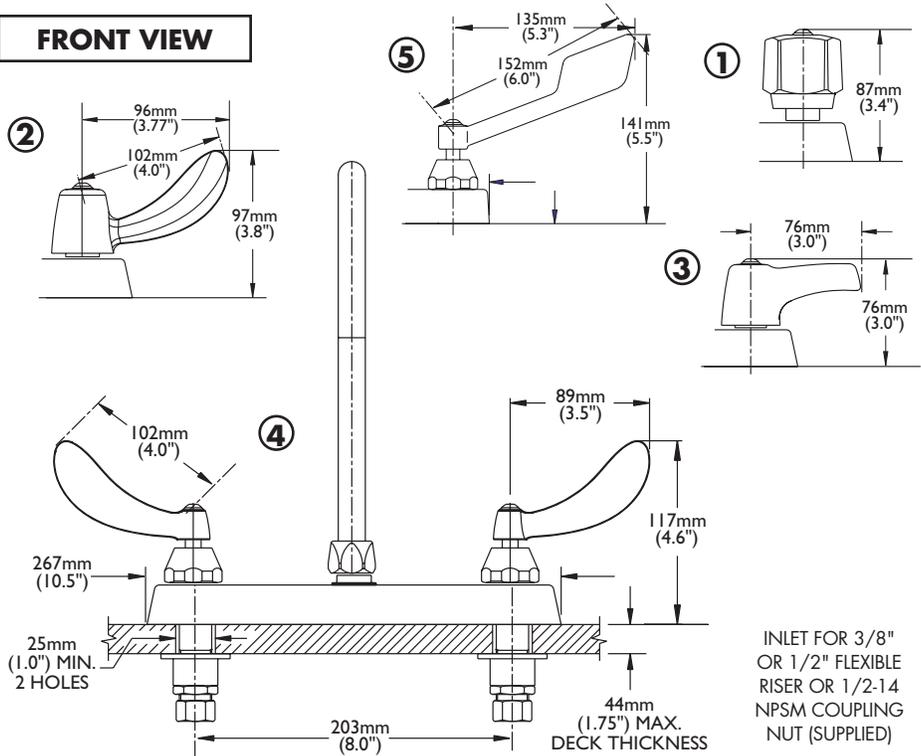
INLET FOR 3/8" OR 1/2" FLEXIBLE RISER OR 1/2-14 NPSM COUPLING NUT (SUPPLIED)
