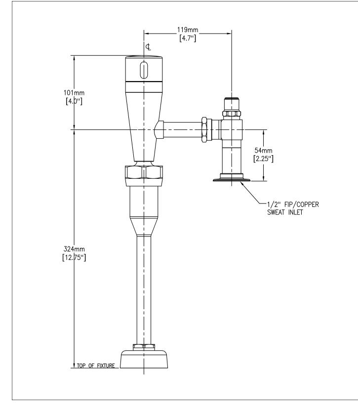
Delta reserves the right (1) to make changes to specifications and materials, and (2) to change or discontinue models, both without notice or obligation. Dimensions are for reference. Measurement may vary plus or minus 6mm(0.25"). Mounting locations are suggested only. Check with local codes for requirements in your area. This spec was produced September 10, 2013.
