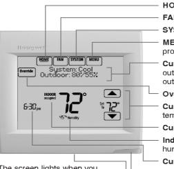
The screen lights when you press any button. It stays lit for 7 seconds after you complete changes. Depending on how your thermostat was installed, the screen light may always be on.
