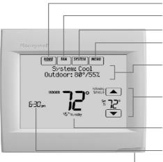
The screen lights when you press any button. It stays lit for 7 seconds after you complete changes. Depending on how your thermostat was installed, the screen light may always be on.
