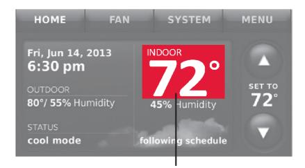
Temperature reading depends on location of sensor
