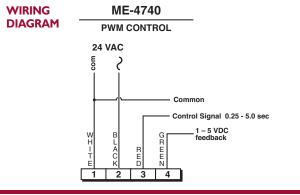
Spartan Peripheral Devices telephone: (450) 424-6067 • fax: (450) 424-6071 • email: info@spartan-pd.com • website: www.spartan-pd.com Zone Valves 4640 4740 4840/44 4940/44 27 February 2012
