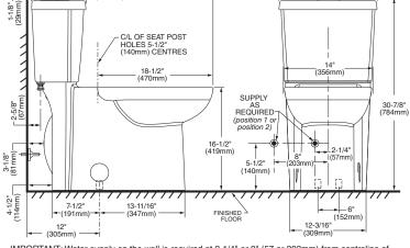
IMPORTANT: Water supply on the wall is required at 2-1/4" or 8" (57 or 203mm) from centreline of the toilet (see rough-in). First suggested position is hidden behind the toilet. The geometry of the toilet gives space for this installation. The second suggested position is next to the toilet. Between these two positions, the space for the supply between wall and toilet is limited to 4-1/2" (114mm). In this case, check your supply and hose dimensions.
