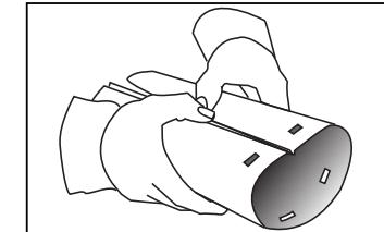
2. Attach vent cap to the pipe
