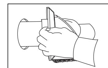
5. Secure the cap to the wall by screwing it into place or caulking around the reveal
