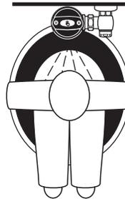
3. When the user steps away from the OPTIMA Plus Sensor, the circuit waits 3 seconds (to prevent false flushing) then initiates an electrical signal that operates the Solenoid. This initiates the flushing cycle to flush the fixture. The Circuit then automatically resets and is ready for the next user.
