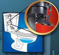
The Leak Sentry® device alerts you to an internal toilet leak and prevents water waste until the flapper is replaced.
