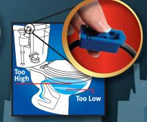
The refill adjuster allows the right amount of water to be delivered to the bowl. Too high a refill to the bowl wastes water down the drain. Too low can cause an improper flush or sewer gas to leak into the room.
