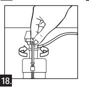
NOTE: Flow from REFILL TUBE must be positioned just above the OVERFLOW PIPE.
