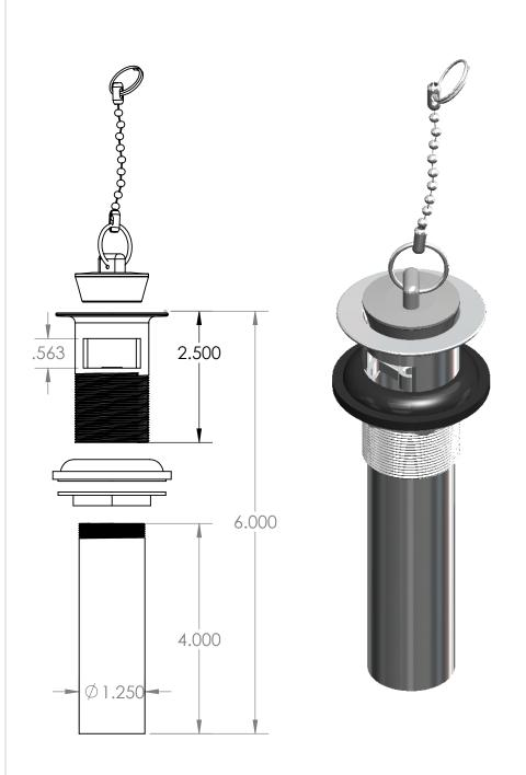
3600-x 1-1/4" 20 GA SEMI-CAST BRASS PLUG & CHAIN P.O. LAV DRAIN
