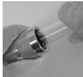
10. Gently push the quartz dome into the gland nut until it touches the top. **Caution:** Do not push hard as it can break the quartz dome.
