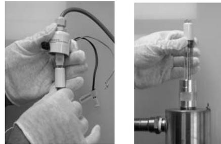
4. Carefully slide UV lamp slightly out of chamber and hold the lamp end with one hand. **CAUTION:** The lamp end can be very hot. Gently pull off the connector with your other hand to disconnect the lamp completely. Slowly remove lamp from the disinfection chamber completely.
