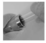
**10.** Gently push the quartz dome into the gland nut until it touches the top. **Caution**: Do not push hard as it can break the quartz dome.
