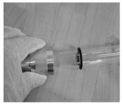
**9.** Replace dome "O" ring on to quartz dome about 1" from the open end.
