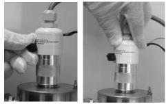
**3.** Loosen the black screw on the lamp connector cover and remove cover from the gland nut.
