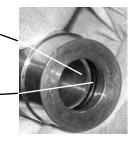
WRONG Quartz dome is NOT past gland nut O-ring (515) and is NOT touching the inside top end of the gland nut.
