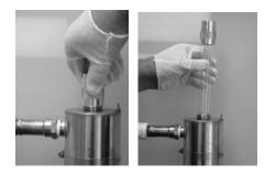
**5.** Remove the quartz dome by loosening the gland nut and carefully extracting from the unit. Remove dome absolutely vertically from its position until the other end comes out. **Caution:** If you bend the dome mid-way, it can break easily and pieces of quartz can fall into the UV chamber. Do not lose the spring that is inside the dome.
