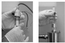
**4.** Carefully slide UV lamp slightly out of chamber and hold the lamp end with one hand. CAUTION: The lamp end can be very hot. Gently pull off the connector with your other hand to disconnect the lamp completely. Slowly remove lamp from the disinfection chamber completely.
