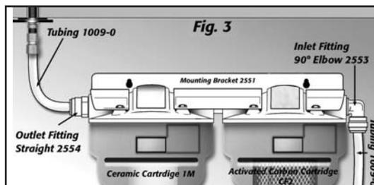
2. Partially screw the 2 mounting bracket screws (1011-0) into screw locations (See Fig. 3). Install mounting bracket and head assembly over screw heads and tighten screws.
