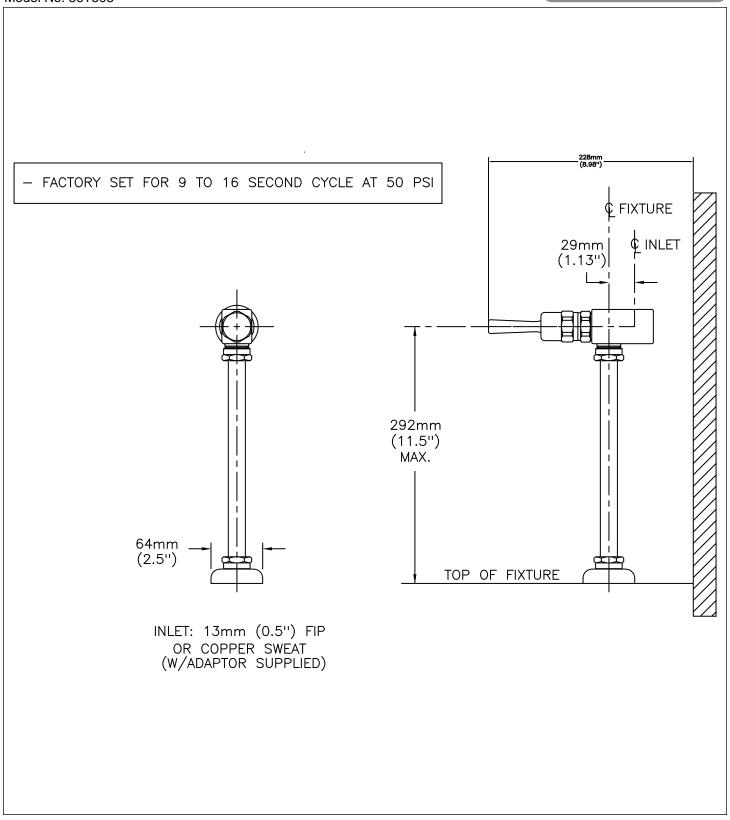
Delta reserves the right (1) to make changes to specifications and materials, and (2) to change or discontinue models, both without notice or obligation. Dimensions are for reference. Measurement may vary plus or minus 6mm(0.25"). Mounting locations are suggested only. Check with local codes for requirements in your area. This spec was produced February 04, 2013.
