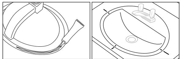
**6** Install supply lines (not included) and trap to drain assembly (not included) as per manufacturers instructions.
