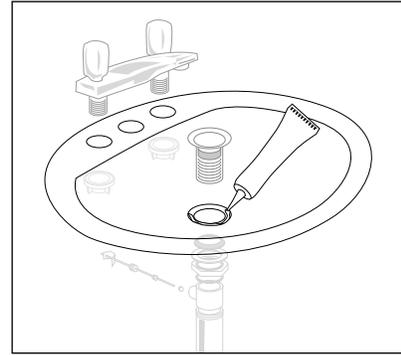
**4** Place the lavatory into the opening in the countertop to check for position, clearance, alignment and fit. Mark the lavatory and countertop with grease pencil to identify the correct position.
