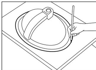
**2** Using a drill create a clearance hole 1/2" ("A" on illustration) inside the outline of the lavatory on the countertop. Using a saber saw cut an opening 1/2" ("A" on illustration) inside the outline of the lavatory starting at the clearance hole.
