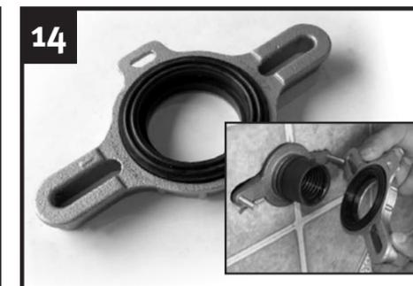
Place the seal into the flange with the ribs facing out. Install the flange with washers and hex nuts, but do not tighten completely.
