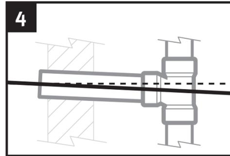
If standing water is present, adjust drain to achieve pitch (code requires 1/4" drop per foot of drain line for proper pitch). Seal the wall according to code.
