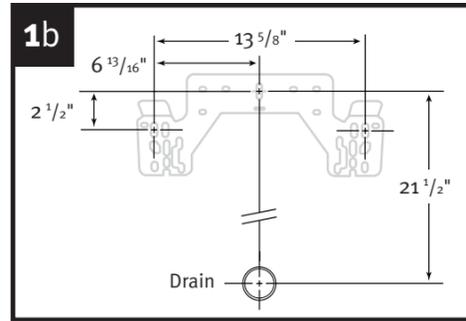
Carrier stud placement: If using in-wall carrier, set bearing rods as shown above.
