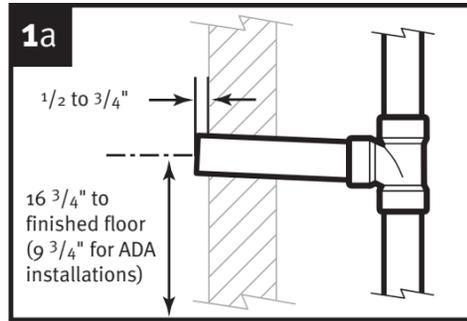
Set drain line height at 16 3/4" from finished floor (standard 24" rim) or 9 3/4" for ADA installation. Threaded nipple should extend 1/2 to 3/4" from wall.
