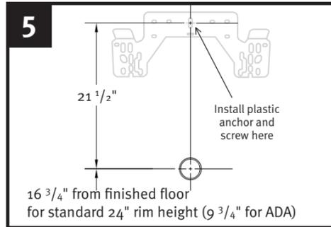
If in-wall carrier is not used, measure and mark the rough-in. Use a 5/16" masonry bit to drill hole, then install the hanger bracket with one plastic anchor and screw.
