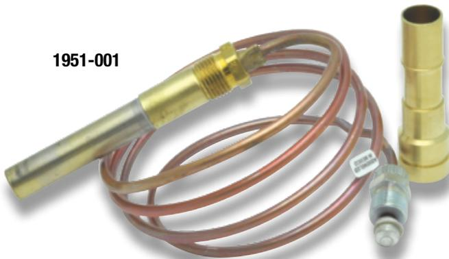
Robertshaw® thermopiles are the industry leader for gas appliance applications. Their primary function is to ensure a standing pilot light is operative so that on a call for heat, the main burner gas will be properly ignited. Thermopiles are placed in gas applications to detect the existence of a flame for safety purposes by shutting off the potential gas flow to a burner.
