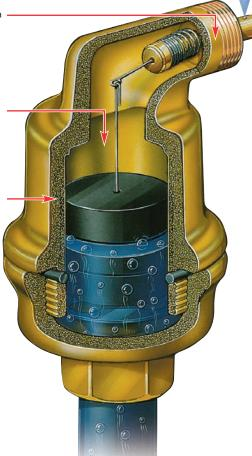
An automatic air vent will only remove free air. Contact your local Spirotherm representative for more information on the Spirovent® air eliminator.
