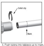
4. Push tubing into taliplece up to mark5. Insert collet clip.
