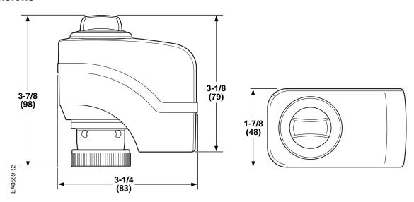
Figure 10. Dimensions shown in inches (millimeters).
