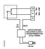
Figure 8. Wiring diagram for SSB81U.
