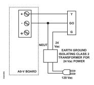
Figure 7. Wiring diagram for SSB61U.
