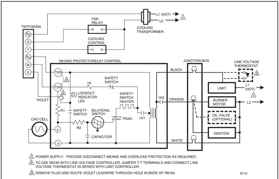
Fig. 1—Typical hookup for Tradeline R8184G with indicator light and isolated alarm relay.
