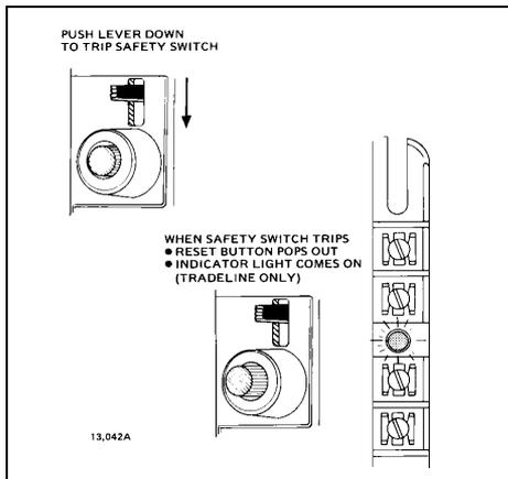
**Fig. 3—Move lever down to trip safety switch.**
