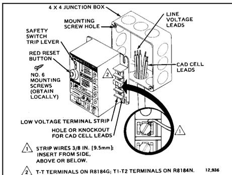
**Fig. 2—Mount the control after connecting line voltage leads.**
