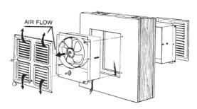
Cut a hole in the wall 8.5" x 9" using telescoping sleeve for the cutting in desired area of the wall between studs or ceiling joists.
