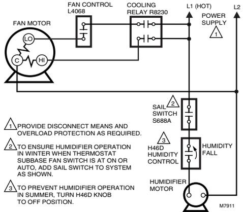
Fig. 5. Typical wiring diagram for H46D in forced air system with 2-speed fan motor.
