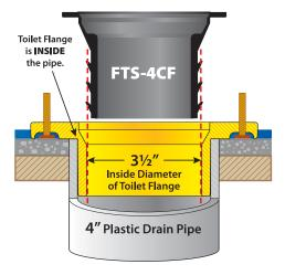
The **FTS-4CF** Wax Free Toilet Seal seals to the 3½" inside diameter of plastic toilet flanges installed inside 4" plastic drain pipe. These flanges are sometimes referred to as a Combination Flange, Slab Flange, or 4x3 Flange.
