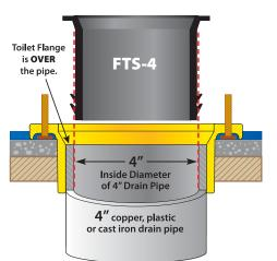
The **FTS-4** Wax Free Toilet Seal seals to the 4" inside diameter of 4" plastic, copper or cast iron drain pipe on both floor mounted and back outlet toilets. Including smooth wall 4" wall carrier models.
