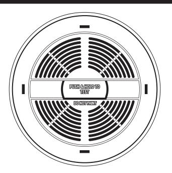
The American Sensors ESA5011, 120 Volt hardwire smoke alarm with built-in relay is an all purpose smoke alarm incorporating "dual-ionization" technology for sensing visible and invisible particles of combustion. The built-in relay allows auxiliary devices to be signalled in an alarm condition, and the unit and contacts will automatically reset upon conclusion. Up to 18 units can be interconnected for simultaneous warnings.
