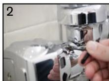
2 Secure the mounting clamp (two screws)
