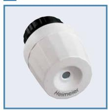
The EMOtec thermal actuator is a twopoint actuator for connection to a temperature controller with two-point output, e.g. HEIMEIER room Thermostat P or Radiocontrol F-System for floor heating.
