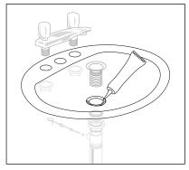
Add a bead of silicone adhesive to rim of lavatory after checking fit and position within the open area of the countertop.
