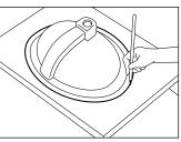
Using a saber saw cut an opening 1-1/2" ("A" on illustration) inside the outline of the lavatory.
