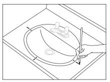
Place sealant on the underside of the lavatory and replace the unit into the cutout area of the countertop carefully aligning with marks made in step 4. Allow sealant to harden.
