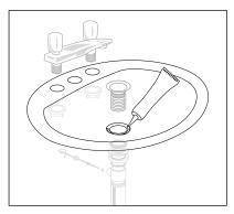
Place the lavatory into the opening in the countertop to check for position, clearance, alignment and fit. Mark the lavatory and countertop with grease pencil to identify the correct position.
